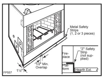
Fig. 14 Safety strip installation.
